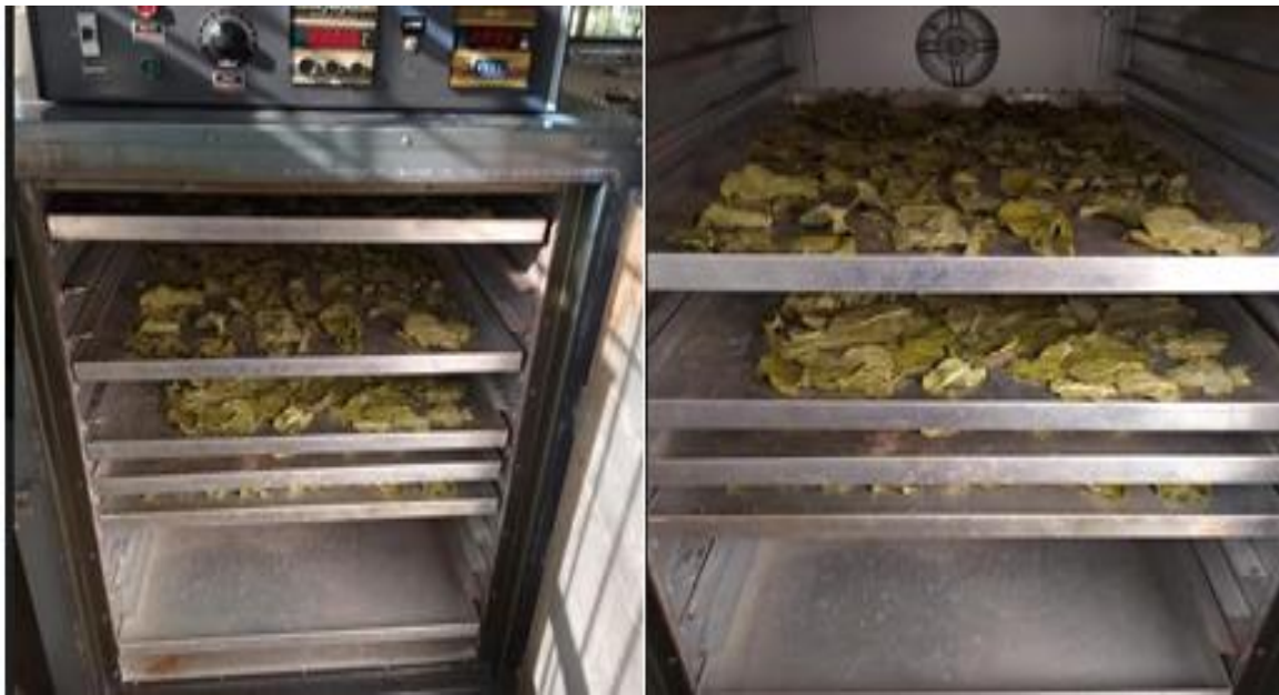
Figure2. Tray Dryer for drying plant material.
