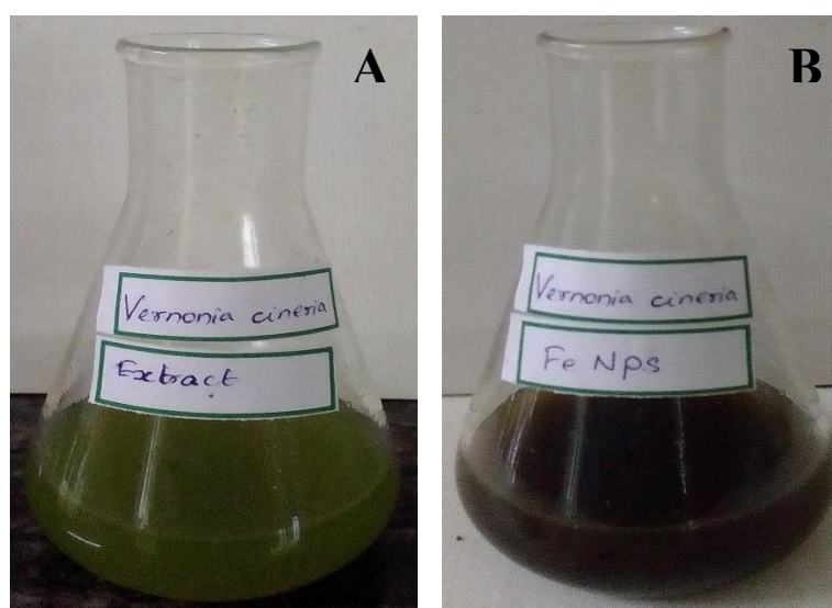
Fig. 3.1: Colour change of the reaction mixture from green to reddish brown indicates the formation of NPs (A) Aqueous V. cinerea extract; (B) Biosynthesized FeNPs suspension (dark reddish brown)
