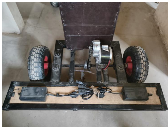
Fig 4: Real Image of Transmission system
