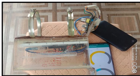
Figure 5: Real time exhaust gas sensing device
