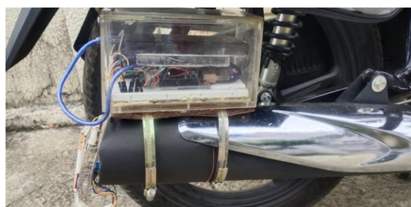
Figure 6: Mounting of exhaust emission sensing device on two-wheeler tailpipe .
