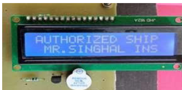
Fig.7.b) LCD displaying authorized ship message
