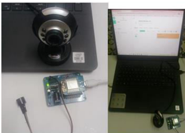
Fig 11 Hardware Setup for IoT integration using Node MCU and PC
