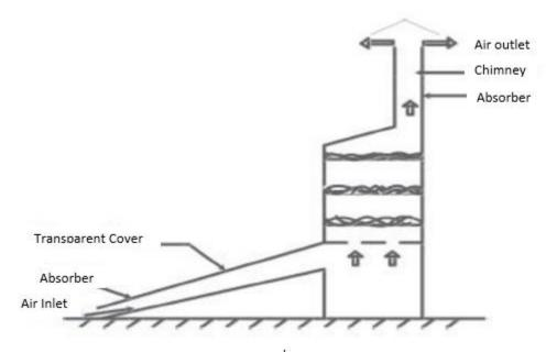
Figure 2: Illustrates the schematic diagram of indirect solar heater.
