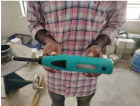
Fig. 1 Rebound Hammer Test (Schmidt's)
