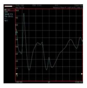
Fig.8 Measured result of vswr plot of the antenna
