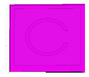
fig1:meta surface unit cell of SRR.
