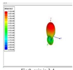
Fig.9 gain in 3-d The peak gain values of metamaterial Triangular shape antenna with 8.4183db
