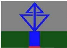
Fig.3 Schematic diagram of the proposed antenna patch without reflector
