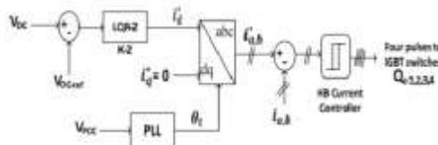
Fig. 6. Control Blocks for the GSI.
