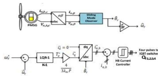
Fig. 5. Control blocks for the MSC.
