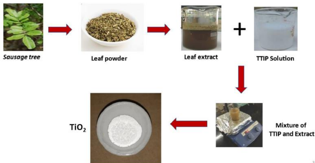
Fig. 2. Diagrammatic representations for Synthesis of TiO 2 NPs.
