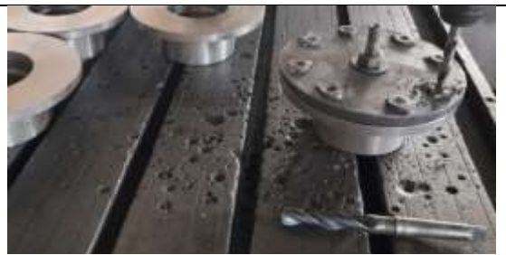
Figure 3. Pilot drilling of the flange using template jig
