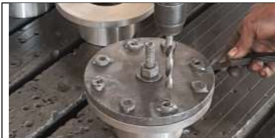
Figure 2. Inspection of flange seating with template jig
