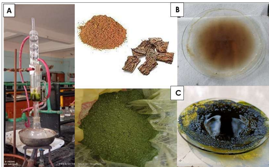
Fig. 2 A. Soxlet extraction, B. Stem extract, C. Leaves extract
