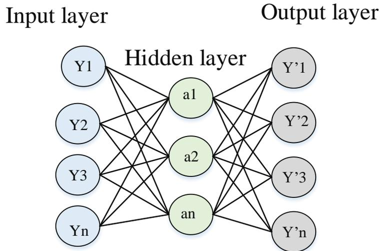
**Figure 3:** Structure of AE
