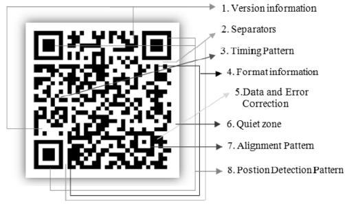
Source : https://www.researchgate.net/figure/Structure-of-QR-Code\_fig1\_275650586
