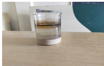
Fig 3.1 photo image of typical Mn-O 2 precipitation after the reduction process
