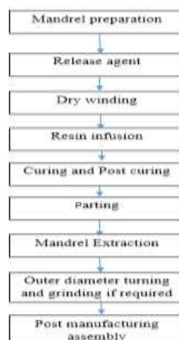
Figure 2.1: Steps used in manufacturing of filament wound product
