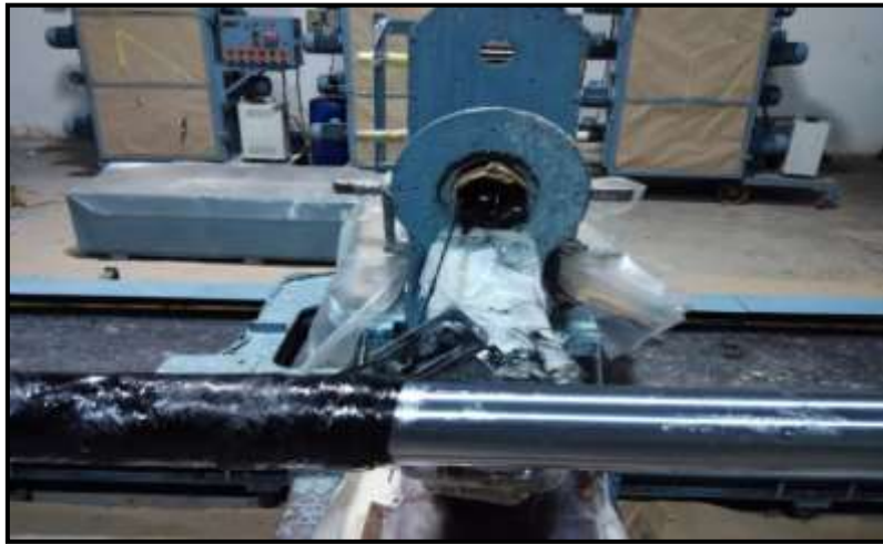
Figure 2.4: Creating fiberglass drive shaft (b)
