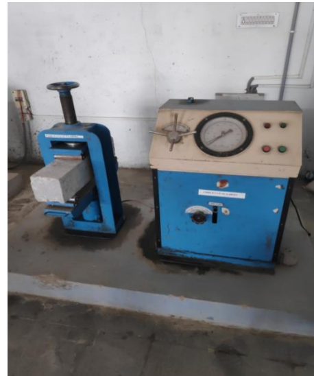
Fig 4.5: Flexural strength testing machine
