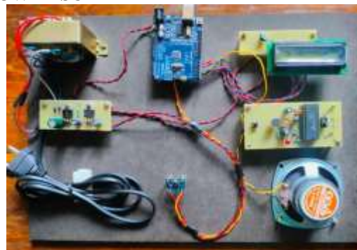
Figure 5: Earthquake detector without power supply
