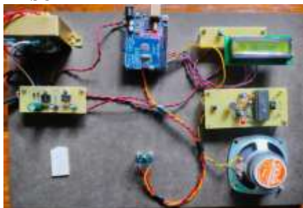
Figure 6 :Earthquake Detector with power supply
