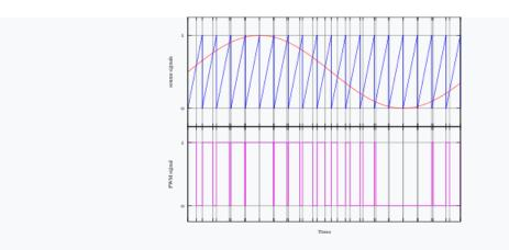
Fig.2: A simple method to generate the PWM pulse train corresponding to a given signal is the intersective PWM: the signal (here the red sine wave) is compared with a sawtooth waveform (blue). When the latter is less than the former, the PWM signal (magenta) is in high state (1). Otherwise it is in the low state (0).
