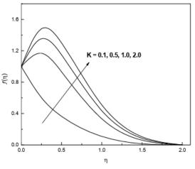
Fig.4. Velocity profiles for different values of K.
