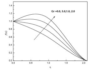
Fig.1. Velocity profiles for different values of Gr.
