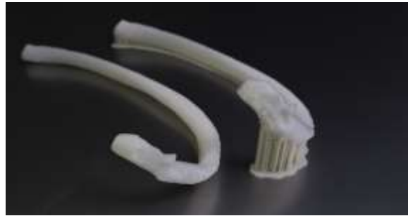
Fig.3 3D printed rib bone without and with support structures
