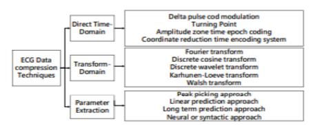
FIGURE. 2 The overview of ECG compression technique
