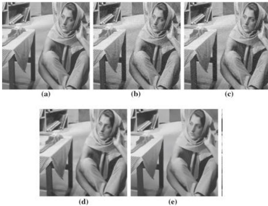
Fig. 3 Visual results of different denoising algorithms for Barbara image (a) Noise free image (b) Noisy image ( \sigma_N = 20 , PSNR = 22.13 dB) (c) Wavelet result, PSNR = 27.08 dB (d) Ridgelet result, PSNR = 28.24 dB (e) Curvelet result, PSNR = 28.11 dB
