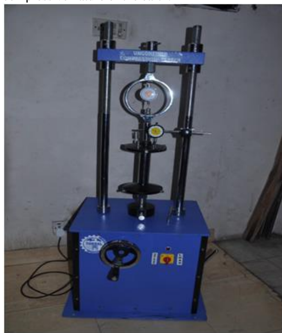
Fig6: Unconfined Compression Testing Machine
