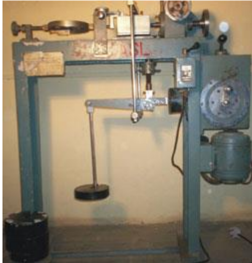
Fig7: Direct Shear Test Apparatus
