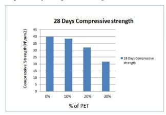
Table 5.6: Test results of Replacement of Fine Aggregate with PET
