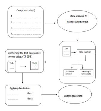
.We can see by the above block Diagram how the process for the classification takes place in the algorithm. The first block specifies the complaints received by the students from a college institution and storing them as Data setfor further processes. The second one specifies the processes of Data analysis such as what type of data is provided and how it should be processed for the next stage and feature engineering.
