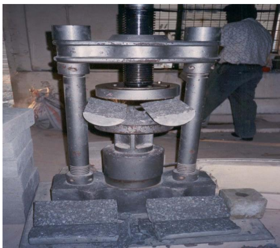
Fig 3.5.2 Split tensile strength for cylinders
