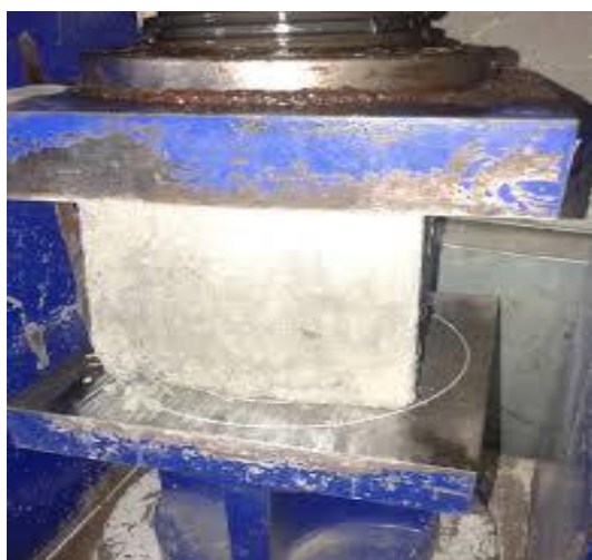
Fig 3.5.1 Compressive strength testing machine After the required period of curing specimens are removed from the curing tank just before testing
