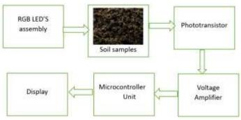
Fig 1: Block diagram
