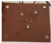
Fig. 2: RGB LED's and Phototransistor arrangements
