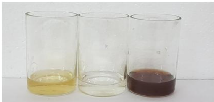
Fig 1: Visual observation (A) P.rubra flower extract (B) AgNO 3 solution (C) Synthesized AgNPs
