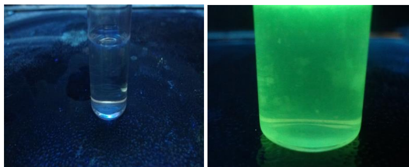
Figure. 2 Photograph of compound h at 0% and 98% \text{H}_2\text{O} fraction in long UV-light
