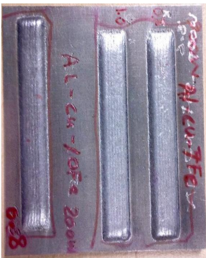
Fig.1: Deposited Al-Cu-Fe Coating Tracks On the Titanium Substrate
