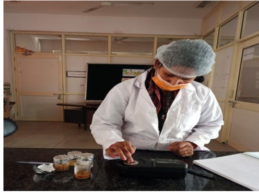
Fig. 4. T.S.S. value of samples determined by hand refractometer
