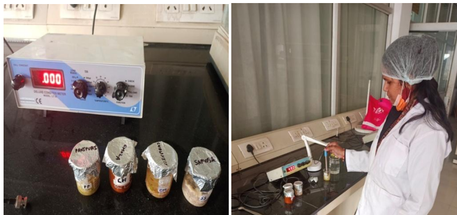
Fig. 3. pH value of samples determined by pH meter
