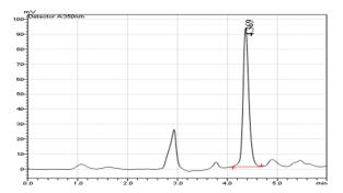
Fig. 6. HPLC Chromatogram for SC-CO<sub>2</sub> extraction of rutin at 50 °C, 200 bar and 80 min
