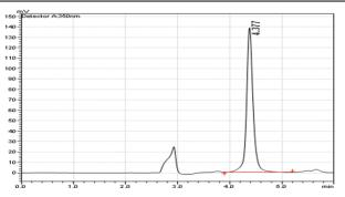
Fig. 4. HPLC Chromatogram for rutin standard (40 ppm)
