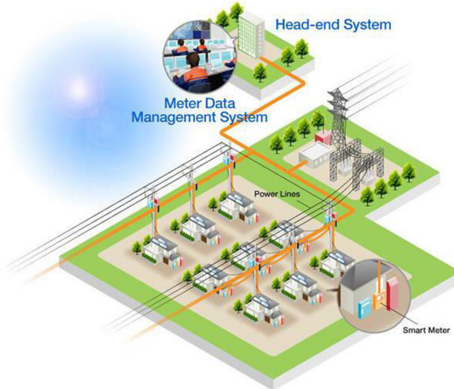
Figure 1. This illustration of a smart metering network includes wireless 2G/3G smart meters
