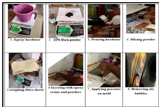
Figure 19 Complete sequential process for fabrication
