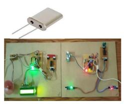
Here, the ERV and non-ERV are displayed in working state where ERV acts as a sender and non-ERV acts as a receiver. In order to replicate the speed of a vehicle, we use a DC motor. The ultrasonic sensor used in this project detects the automatic distance of the nearby vehicle and sends the information to the non-ERV which is displayed on the LCD display.
