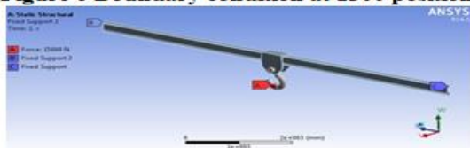
Figure 7 Boundary conditions at 4300 position
