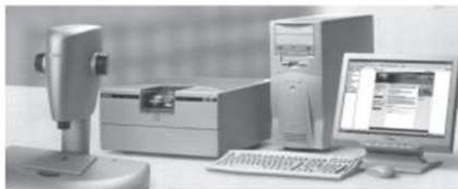
Figure 12. Cerec Scan –integrated laser scanner, dotscanner in the left engine Fig. 13. Cerec inLab system – from left to right: inEos ekstraoral Cerec in Lab with inbuilt dot scanner, PC computer with 3D softver
