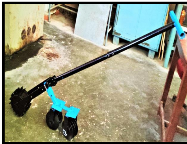
Fig 9: Developed Manual Disc weeder
