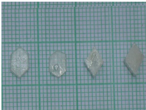
Fig : a. Pure thiourea single crystal and b NaCl doped thiourea single crystals.
