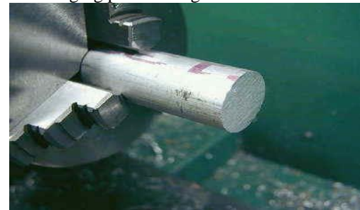
Fig. 2 Fixing of workpiece
