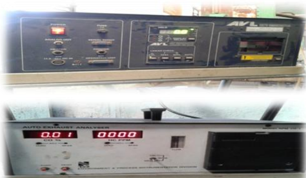
Figure- 3. Exhaust gas analyzer to measure CO, HC& smoke
