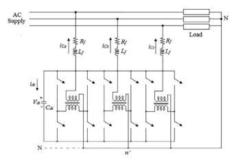
. A distribution line with DSTATCOM connected at PCC
