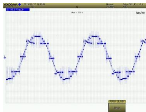
Fig. 10 Output voltage waveform of Inverter
