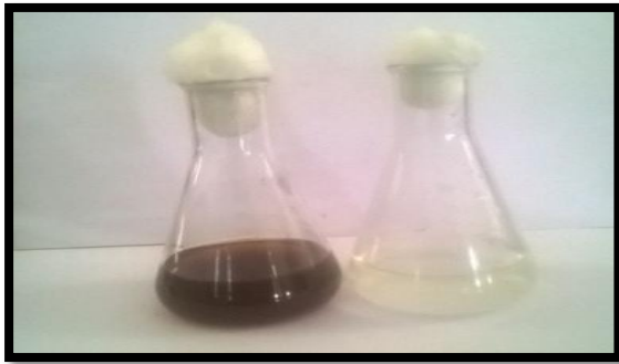
Fig 1. Biosynthesis of AgNPs: Color of solution change from colorless to brown within 24 h Incubation
