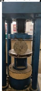
Fig. 2 Evaluating the Split Tensile Strength
