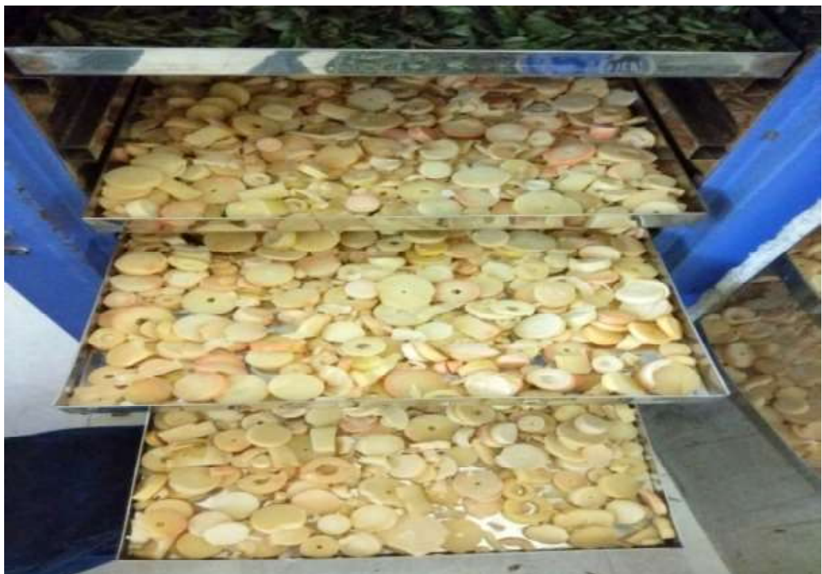
Figure 4: Bamboo Shoot Pieces Spread in Trays, Ready for Tray Drying
