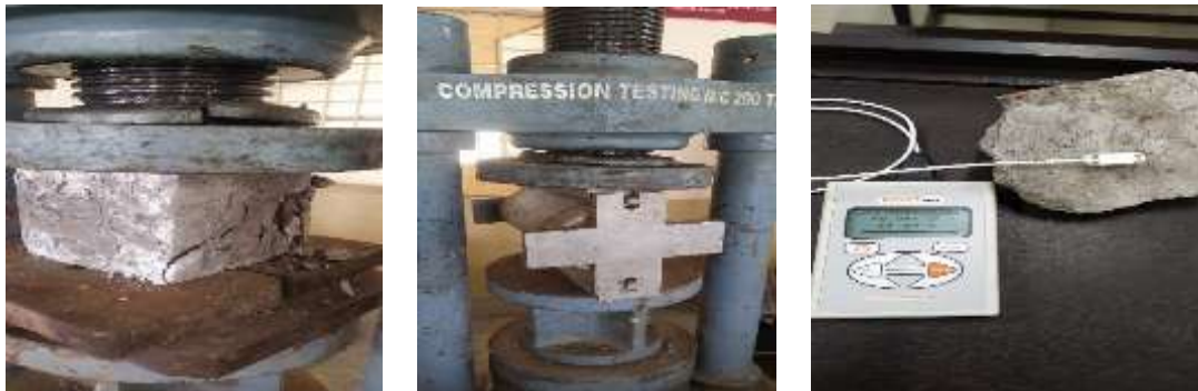
Figure 3.1: Compressive strength of NCC and MCC, Split tensile test for Normal cement concrete and modified cement concrete, Thermal conductivity TC test performance with KD2 Pro Analyzer
