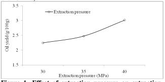
Figure 1- Effect of extraction pressure on extraction yield
