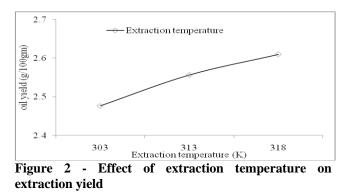
The result showed that at higher pressure, solute vapor pressure increased with temperature compared to solvent vapor pressure. But after 313 the extraction yield was started to decrease due to start of crossover effect which is explained by Said *et.al*,. (2014) in their literature and thermal degradation of volatile compounds as well.
